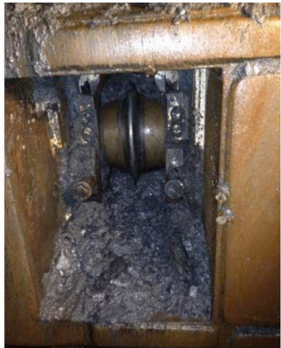
Fig. 20: Classical dry mucking with a hardrock cutterhead (left); clogged hardrock cutterhead after wet mucking through a fault zone (right, taken from a project in Turkey).
